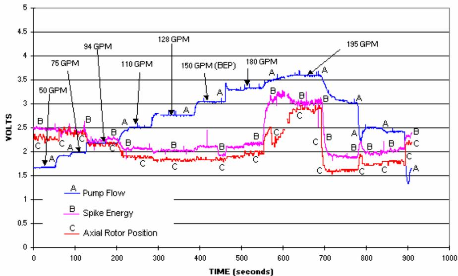
Figure 18. Flow changes (20 GPM increments) [3]
