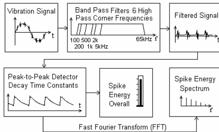
Figure 1. Flow chart of Spike Energy signal processing
