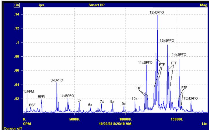
Figure 15. Velocity spectrum of the pump
