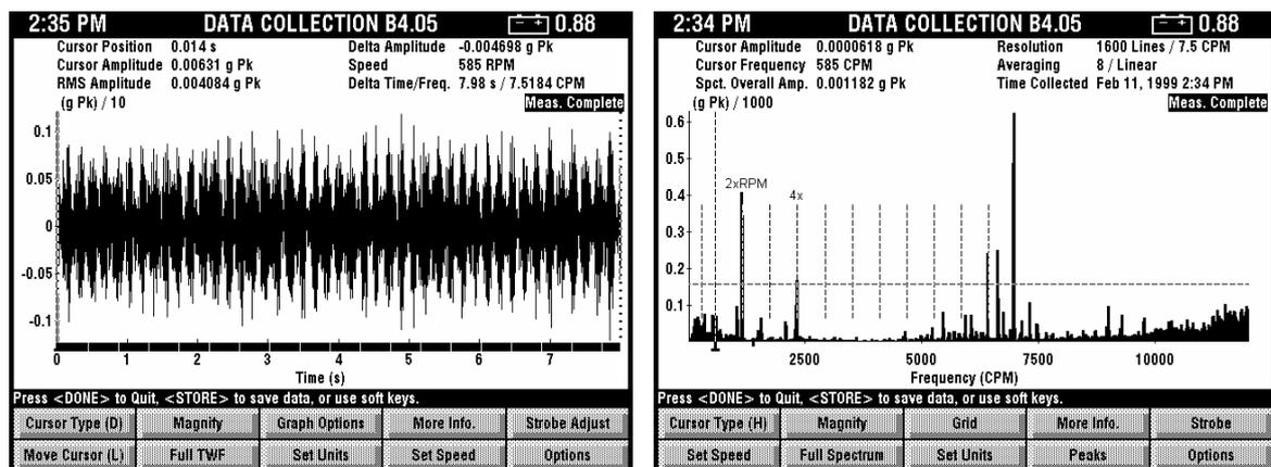
(a). Time waveform (b). Frequency spectrum
