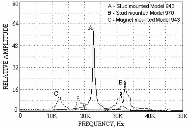
Figure 5. Frequency response of accelerometers [1]
