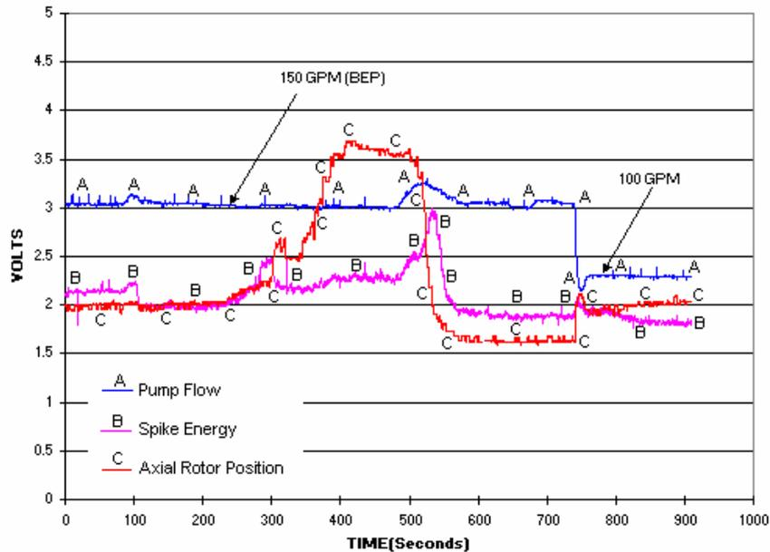
Figure 19. Reduced suction pressure (at constant 150 GPM) [3]
