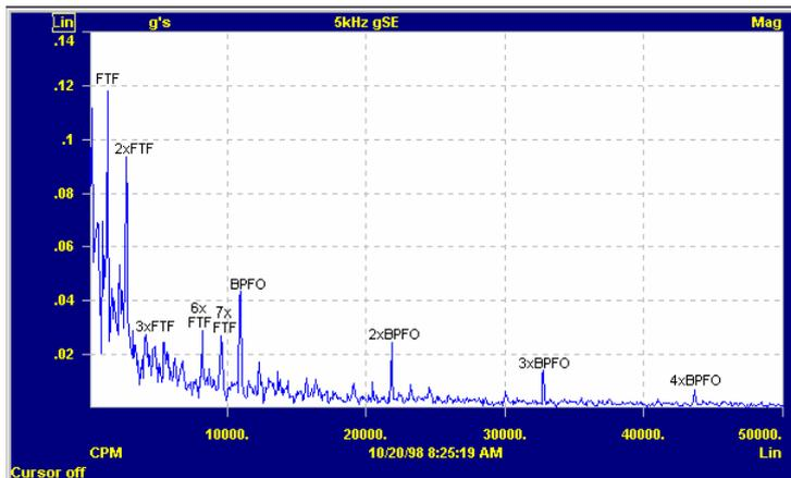
Figure 16. Spike Energy spectrum of the pump
