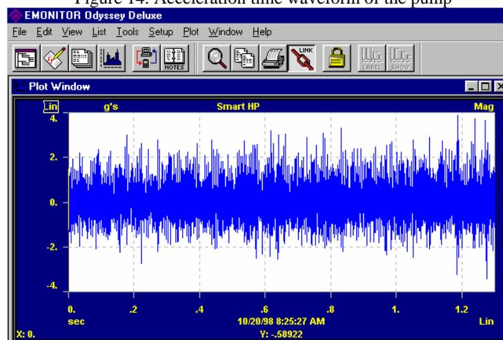
The measured Spike Energy overall was also high at 5.11 gSE indicating high impacts. The pump bearing defect was clearly identifiable in the velocity spectrum and Spike Energy spectrum, as shown in Figure 15 and Figure 16. In the velocity spectrum, the higher order harmonics of ball pass frequency – outer race (BPFO)
