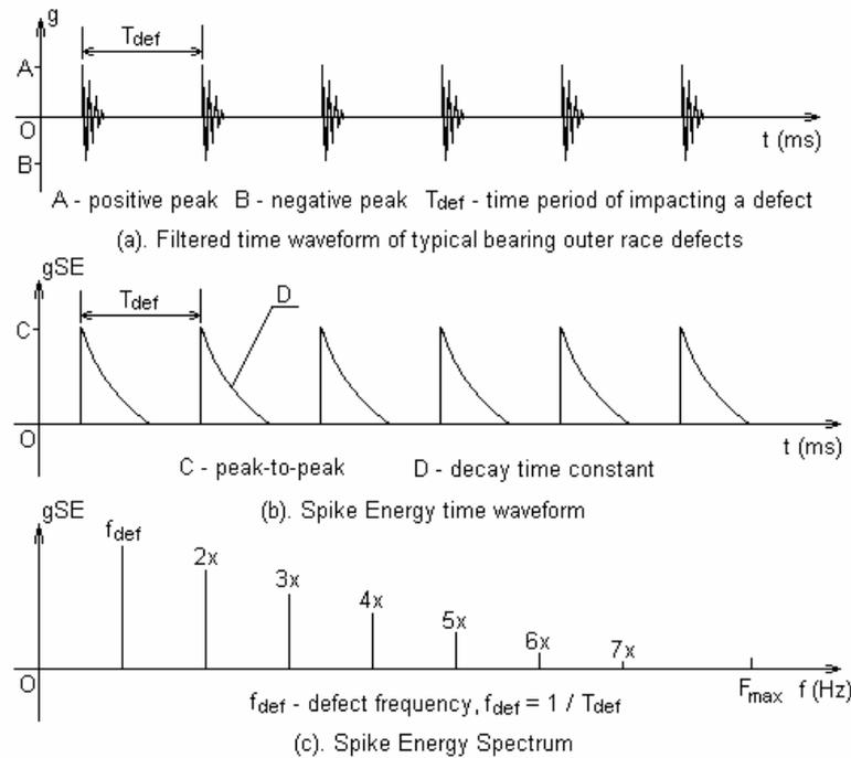
Figure 3. Spike Energy peak-to-peak detection
