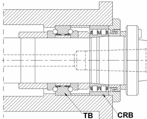
TB – Double direction angular contact thrust ball bearing
