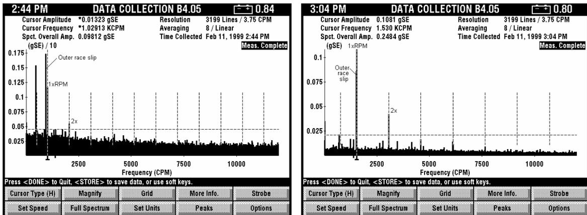
(a). Measured at 1029RPM (b). Measured at 1530RPM
