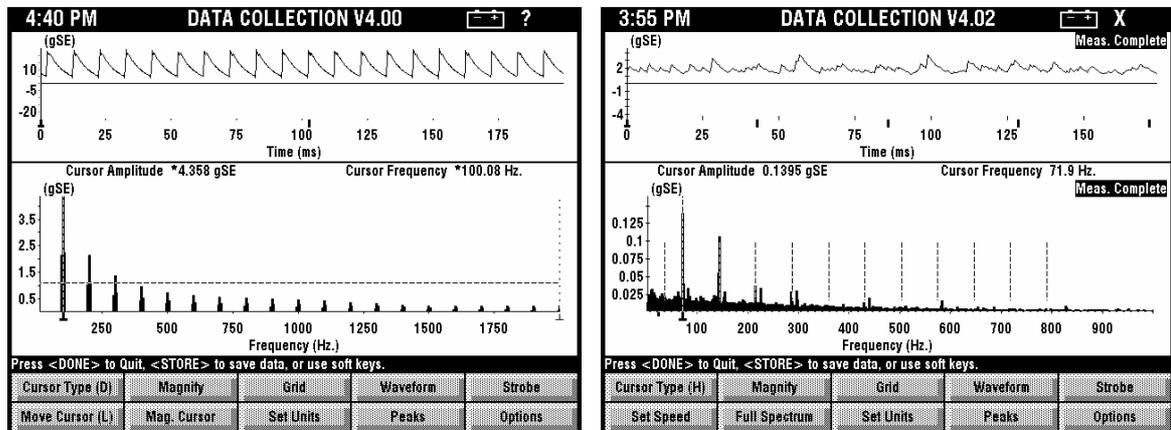
(a). Signal generator data (b). Spindle data
