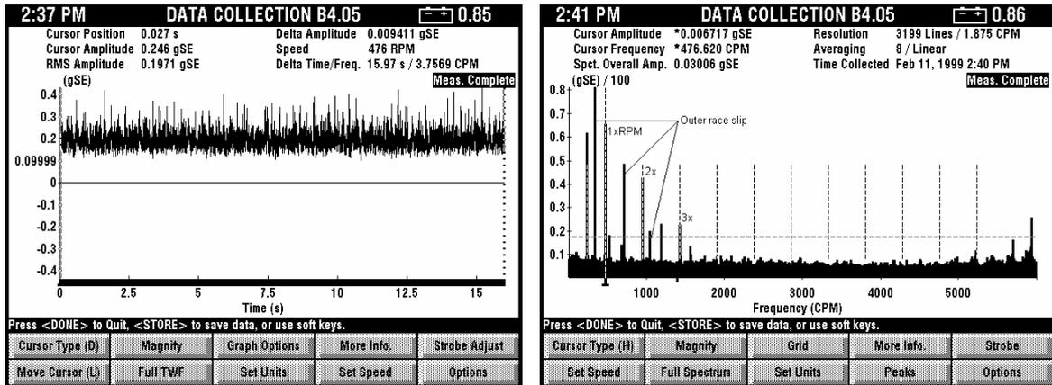
(a). Time waveform (b). Frequency spectrum
