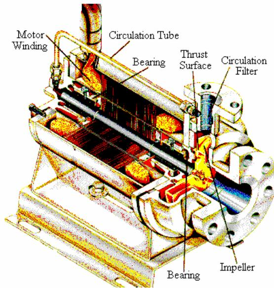
Figure 17. Canned motor design of sealless pump [2]
