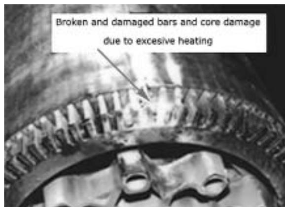
Figure 10. Food Mixer Motor—Broken Rotor Bars.
