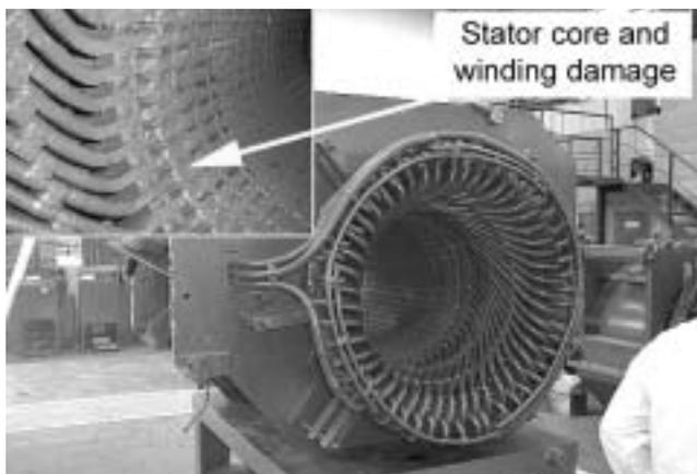
Figure 8. Mechanical Damage to HV Stator Winding.
