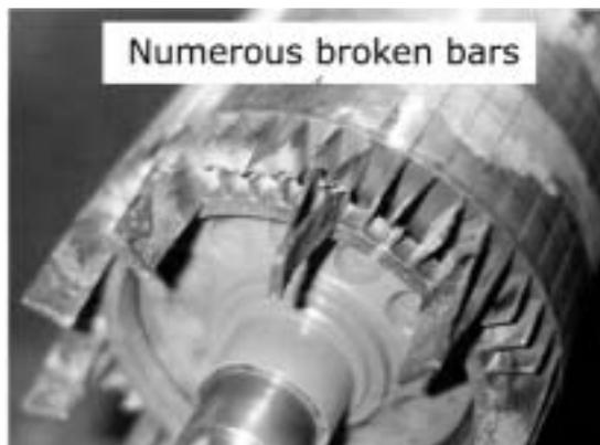
Figure 9. Crane Motor—Broken Rotor Bars.
