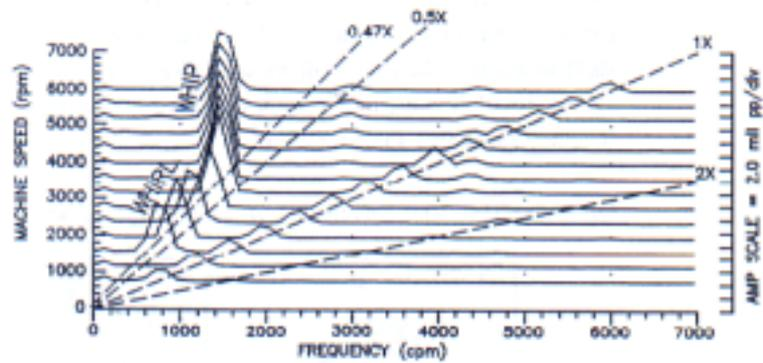
Figure 7 Cascade plot illustrating whirl and whip
