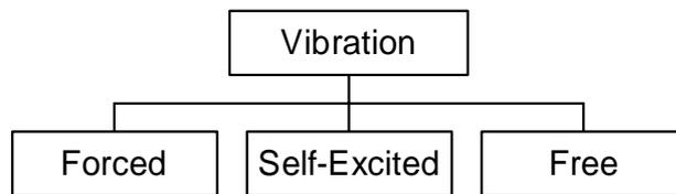
Figure 1 Vibration classes based on source of excitation
