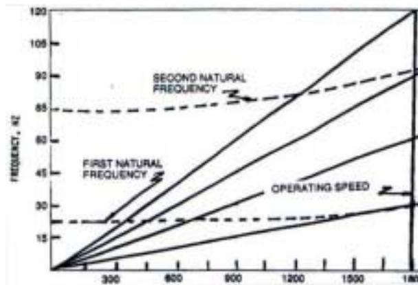
Figure 5 Frequency interference chart
