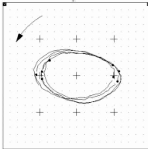
Figure 9 Orbit plot illustrating a fluid induced vibration
