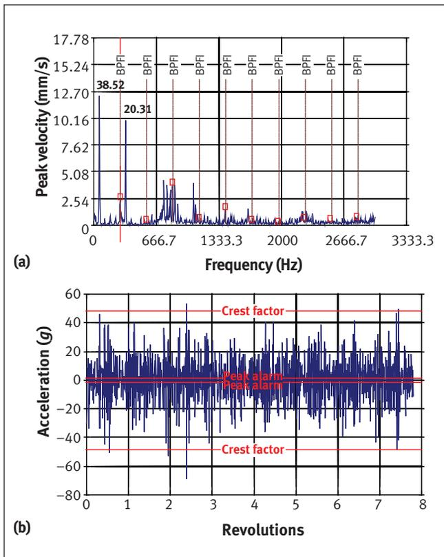
Figure 3. Example 2, information collected from a boiler feed water pump showing: (a) spectrum; (b) time-waveform. Ball pass frequency inner race is indicated as BPFI.
