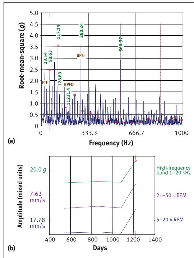
Figure 4. Example 2, information collected from a boiler feed water pump showing: (a) the high-frequency natural bearing resonance indicator; (b) discrete frequency indicator and trends. Fundamental train frequency (FTF), ball pass frequency outer race (BPFO) and ball pass frequency inner race (BPFI) are indicated.
