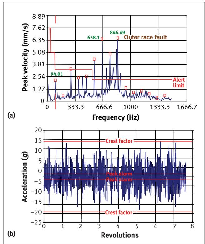
Figure 2. Example 1, information collected from a ballast scrubber pump showing: (a) spectrum; (b) time-waveform.
