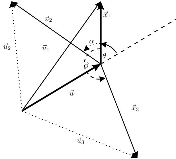
**Figure 1:**  $1 \times$  Vibration Vectors with Three Trial Weights In a Single Plane
